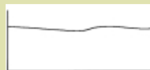
Figure 2: Screw compressors are best where the demand for compressed air is relatively constant, as in a production line situation
