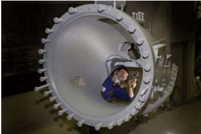
Dean Lewis spray-paints a Hamilton jet boat unit where heat from making compressed air is recaptured to help dry the paint.
